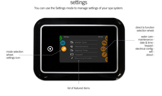
To select the settings mode, slide the left wheel up or down until the settings icon menu is highlighted in the middle.
