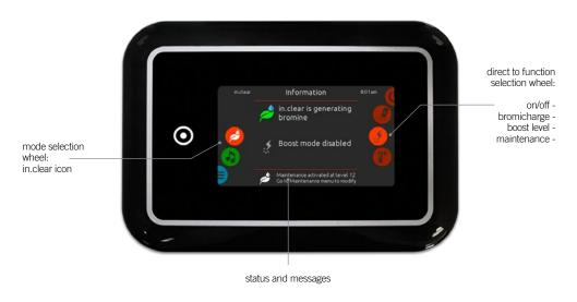
To select the sanitization mode, slide the left wheel up or down until the in.clear icon menu is highlighted in the middle.
