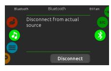
If a device with Bluetooth technology is connected to the in.stream 2, you can disconnect it by pressing the Disconnect key at the bottom of the screen.
