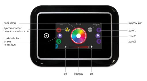
To select the color mode, slide the left wheel up or down until the in.mix icon menu is highlighted in the middle.
